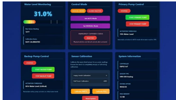
Water level monitoring and pump control.
