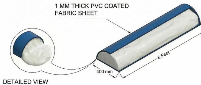
Fig. 7. Flexible Fluid Chamber
