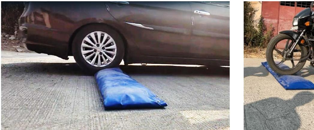
Fig. 7. Deformation of Breaker By 2&4 Wheeler
