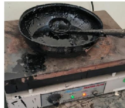
Fig. 4: Heating of Bitumen
