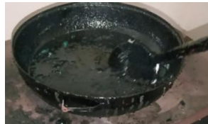
Fig. 5: Mixing of Plastic with Bitumen
