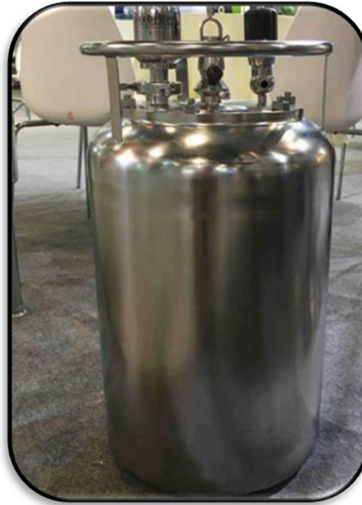
Figure 2: Yeast propagation and pitching vessels used during successive generations of yeast propagation
