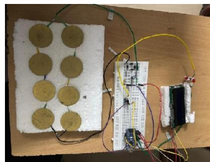
The electrical energy generated by the piezoelectric sensors is initially in alternating current (AC) form. A rectifier circuit is used to convert this AC voltage into direct current (DC). The converted DC voltage is then regulated using a voltage regulator to ensure a stable output suitable for storage and usage. The regulated power is stored in rechargeable batteries or capacitors for later use.
