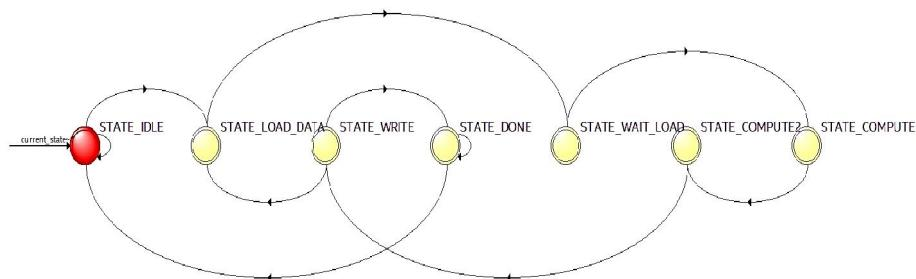
The system architecture consists of an input buffer that forms a 4×4 sliding window of image pixels, a coefficient memory holding fixed kernel values, and a convolution engine performing parallel multiply-accumulate operations. An FSM controller coordinates data loading, computation, and output storage. The pipelined design enables continuous processing of input data with improved throughput.
