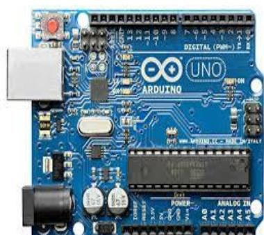
An Arduino microcontroller is proposed as the central control unit for future implementation. It is intended to receive classification results from the CNN model and control the bin rotation mechanism. Its low cost, simplicity, and ease of programming make it suitable for automated waste segregation applications.
