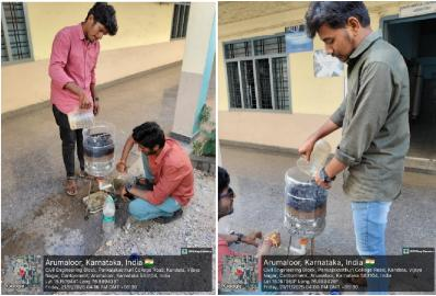
Raw river water was gently poured into the top of the bed filter and allowed to pass through the filter media under gravity flow conditions. The water sequentially passed through the biochar and sand layers, enabling both adsorption and physical filtration mechanisms. A controlled flow rate was maintained to ensure effective contact between water and filter media. The filtered water was collected at the outlet in clean containers for further analysis.
