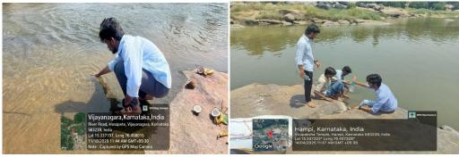
River water samples were collected from an accessible location along the Tungabhadra River using clean, pre-washed plastic containers to avoid contamination. Prior to sample collection, the containers were rinsed with river water. Care was taken to avoid the inclusion of floating debris and sediments. The collected samples were properly labeled with date and location and transported immediately to the laboratory for filtration and analysis.
