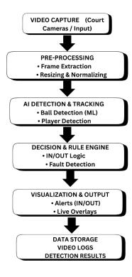
Figure.1. System Architecture
