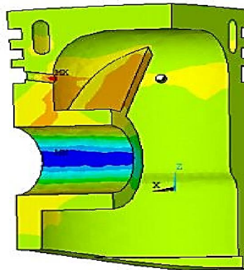
Fig. 5 Thermal Stress Nephogram Within the Piston
