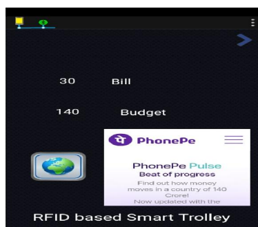
Fig. 4: Virtuino app showing real-time Bill and Budget display.
