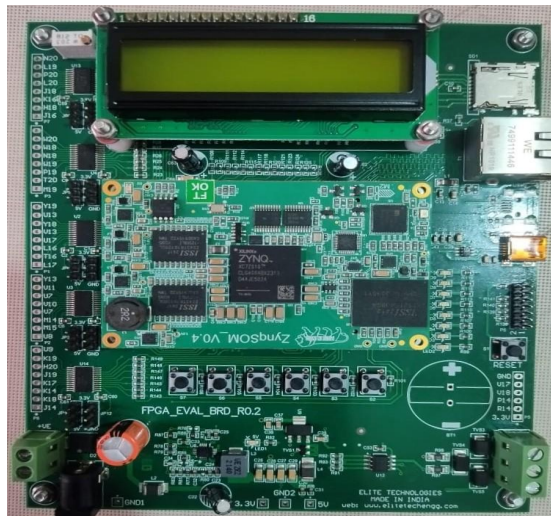
Fig. 3. Fabricated ZEDX hybrid FPGA–ARM evaluation board after assembly
