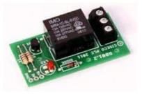
A relay is an electrically operated switch that controls a high- power circuit with a low-power signal. It's essentially a switch that's activated by an electrical current, allowing a small current to control a larger one. This is useful for situations where you need to switch a high-power device, like a motor or a light, with a low-power control signal, such as a button press.
