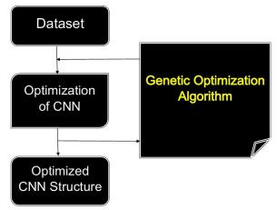
This optimization process is conducted incrementally. It begins by designing an optimal structure for a simple, single-layer CNN using the large-scale FER-2013 dataset. A new convolutional layer is then added to the network, and the entire structure is re-optimized by the genetic algorithm. This sequential, layer-by-layer optimization continues until no further performance improvements are observed, resulting in a highly specialized and effective network architecture.
