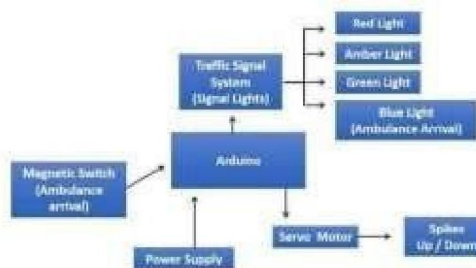
Fig 1: Block Diagram of Advanced Traffic Control System
