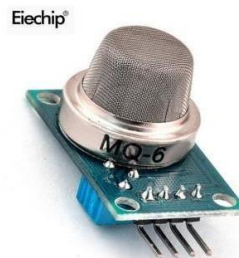
Figure 4: Carbon Monoxide (CO) sensor MQ 6
