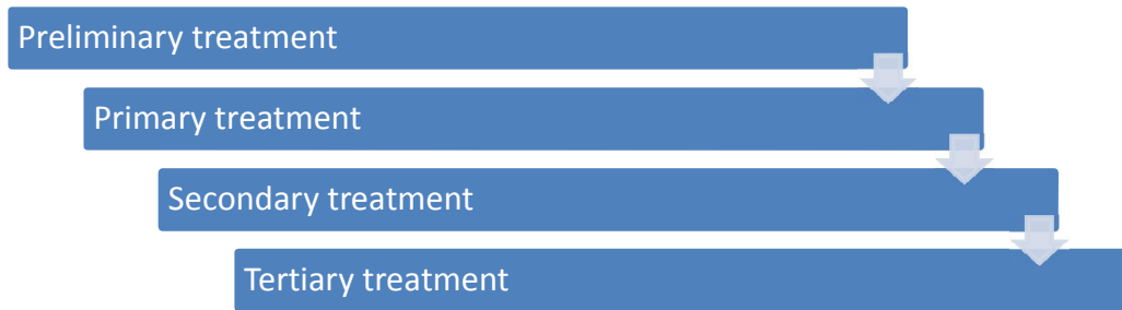
Figure 2. Waste water treatment levels
