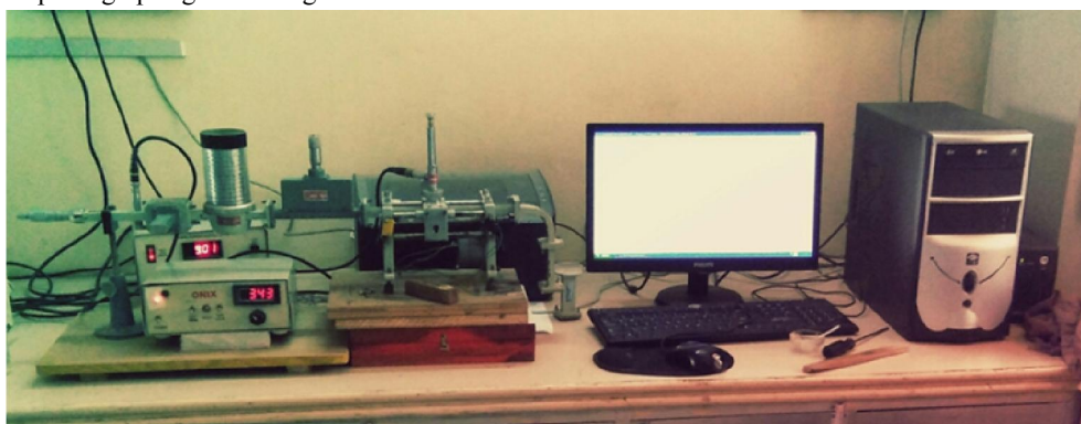
Fig.1 Photograph of automated X-band microwave bench setup for measurement of dielectric constant of contaminated and reclaimed soils.
