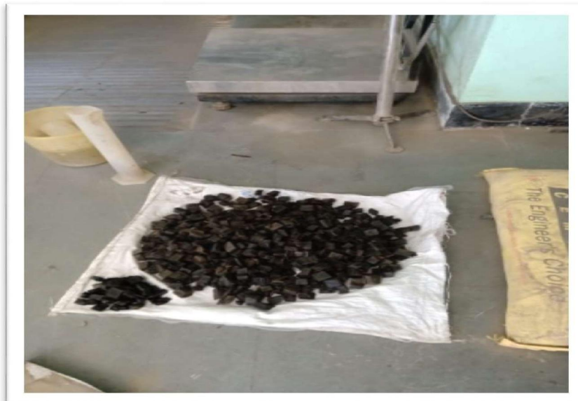
Figure 1. Cutting of waste tyre in Nominal size of Coarse Aggregate
