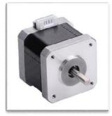
Model: NEMA 17 Step Angle: 1.8° per step Rated Voltage: 2.8V to 4.8V Current per Phase: 1.2A to 2.0A Holding Torque: 40 N · cm Number of Phases: 2 Resistance per Phase: 1.1–2.2 ohms Inductance per Phase: 2.8–4.5 mH Shaft Diameter: 5 mm Connector Type: JST-PH 4-pin Motor Frame Size: 42 mm × 42 mm
