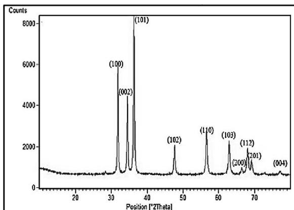
Fig. 1 XRD pattern of ZnO nanoparticles.
