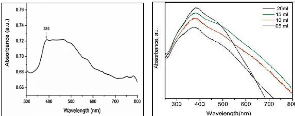
Fig.9 UV-Vis. Spectra of ZnO nanoparticles fig. 10 UV-Vis. Spectra of CuO nanoparticles
