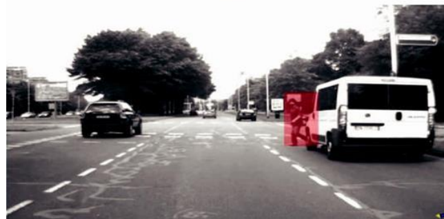
Figure 3: These are two frames of a sequence. (a) The system detects the pedestrian and issues an internal alert but no warning to the driver. (b) When a detection of pedestrian monitors the internal alert, a warning is quickly sent to the driver[1].
