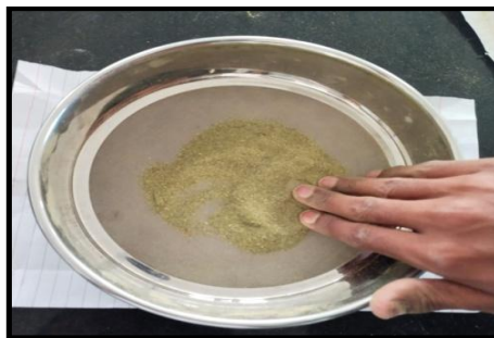
Fig.5 – Passing through No.40-mesh sieve
