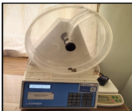
Fig.12 – Fraibility Test for tablet
