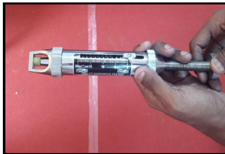
Fig.11 – Hardness test for tablet
