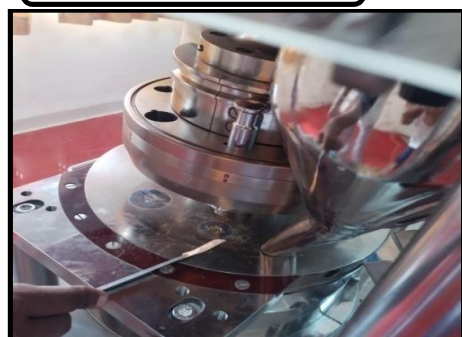
Fig. 9 – Filling the die with the blended powder
