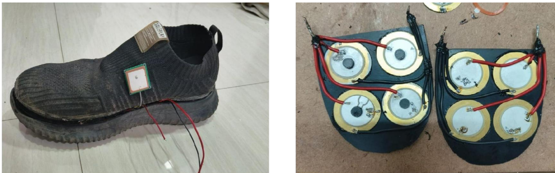
Figure 7. Piezo Discs Arrangement in real shoes
