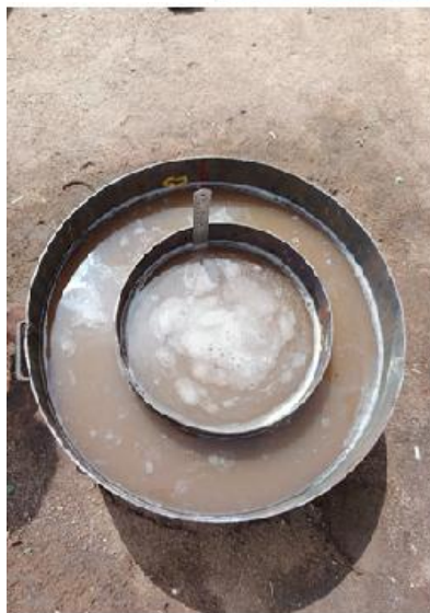
Adding water to both inner and outer rings
