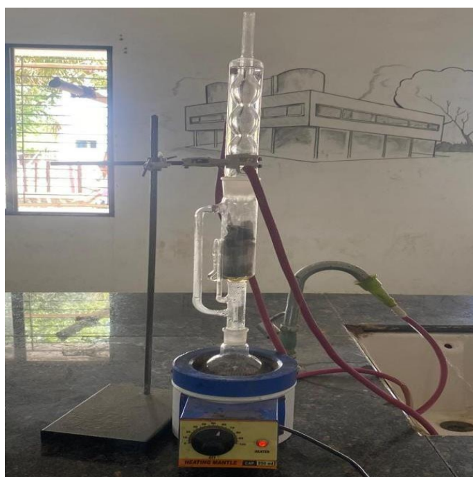
Fig. Schematic of a Soxhlet extraction apparatus indicating the vapor and liquid extractant . paths. The sample under extraction is cushioned by loosely packed ceramic fibers.
