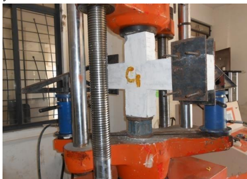
Fig.2 Testing of Beams –Column Joint
