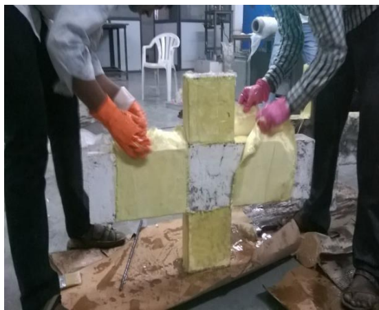
Fig.1 Fixing Aramid Sheet on Beam-Column Joint
