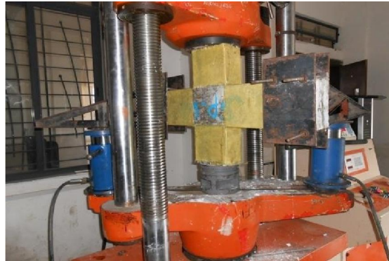
Fig.3 Test setup for wrapping Beam-Column Joint specimen
