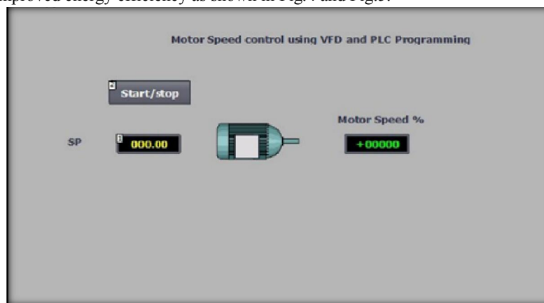
Fig. 4 Frequency set at 0 Hz through HMI for the motor speed control at 0 rpm
