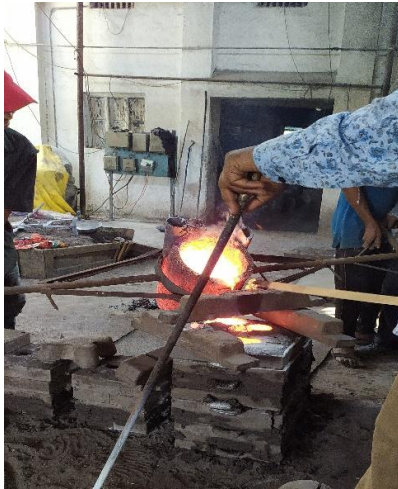
Figure 4: Pouring of molten metal in moulds
