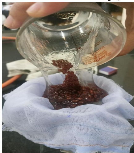
Fig .06 Extraction of Flaxseed Mucilage (filtration)
