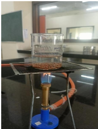
Fig .05 Extraction of Flaxseed Mucilage ( Boiling)
