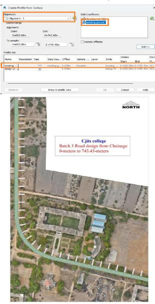
Create Design Profile Design Profile Creation: Once the existing ground profile is created, you can create a proposed profile for your road. Go to Home → Create Design → Profile → Profile Creation Tools. Select your alignment and click on Create Profile View to generate a new profile view. Define vertical curves, grades, and elevations for the proposed design profile. Adjust slopes and curves for smooth transitions, including vertical curves to meet design standards
