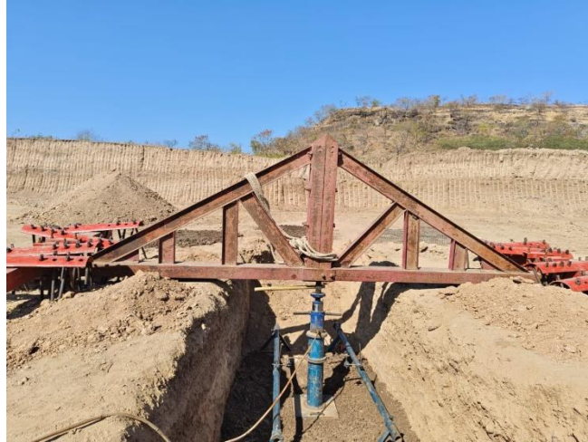
Figure 2: Plate Load Test Setup
