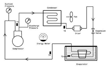
The major components used in the ice plant are described in the subsequent sections:
