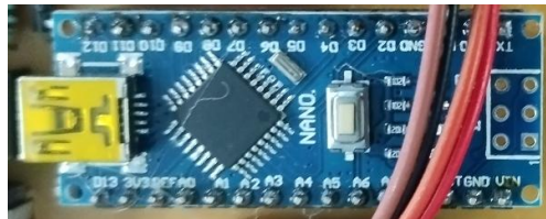
Figure 3: Arduino Nano working as a Boost Converter
