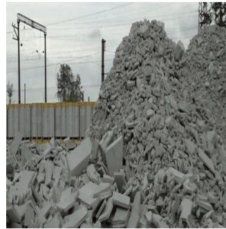
Fig 1 CLC Waste Block
