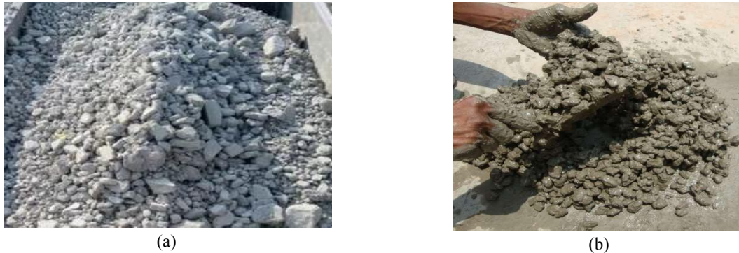
Fig 3. a) Collection of Crushed Waste CLC Blocks b) Coated with a 1: 4 cement slurry
