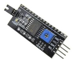
The I2C (Inter-Integrated Circuit) Module is a communication interface that allows multiple devices (like sensors and displays) to connect to a microcontroller (like Raspberry Pi) using only two wires — one for data (SDA) and one for clock (SCL).
