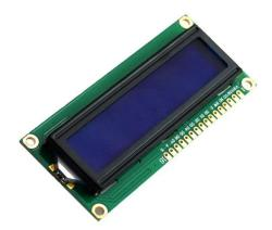
The LCD 16x2 is a widely used alphanumeric display module that can show 16 characters per line across 2 lines. It is a simple and cost-effective display that can easily interface with microcontrollers like the Raspberry Pi.
