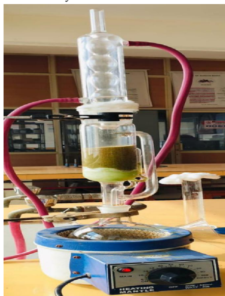
Fig : Soxhlet extraction of leaves of plant and extract of leaves .
