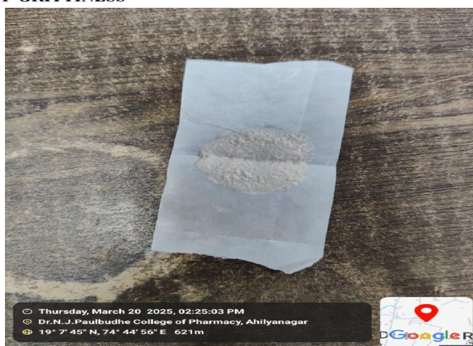
Fig 9 :Determination of Grittiness
