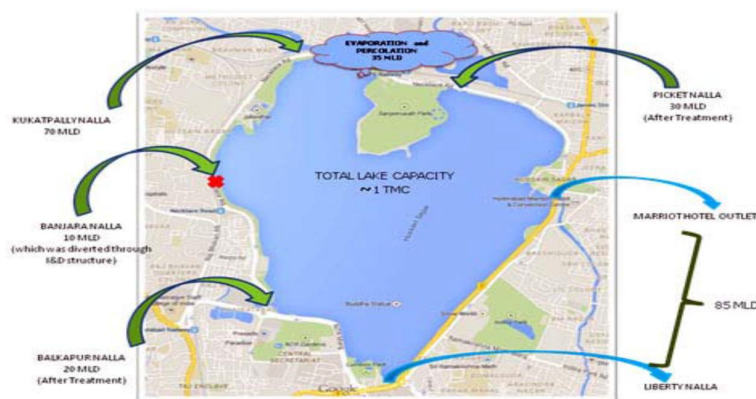
Figure 2: Hydrological balance of the Hussain sagar lake (Source: EPTRI - A Pilot Study on Hussain sagar Lake Environment, March 2015)
