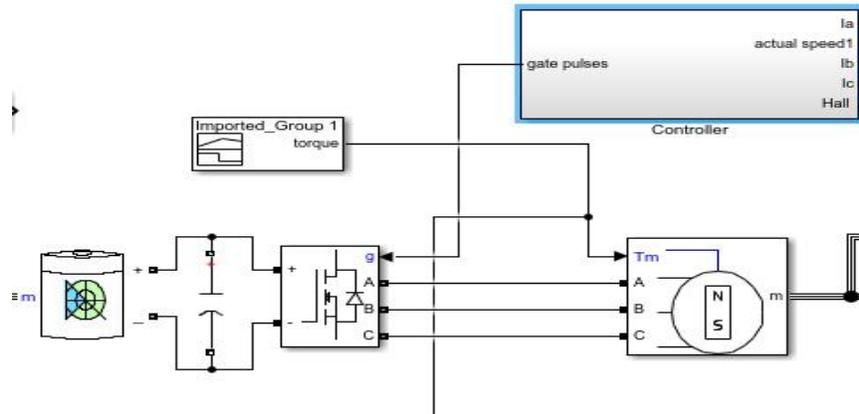
Figure 3 Configuration of Inverter Circuit
