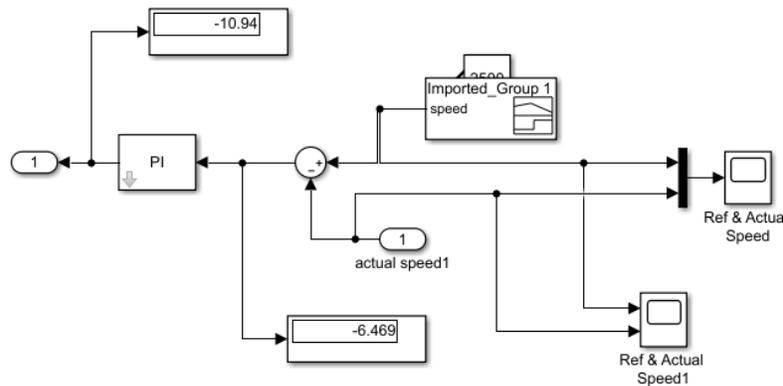
Figure 1. PI Controller of the system
