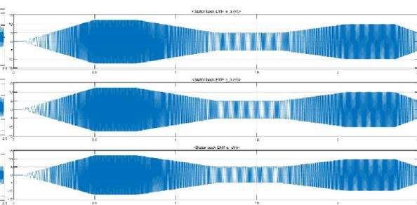
Figure 9: Stator Back EMF waveform
