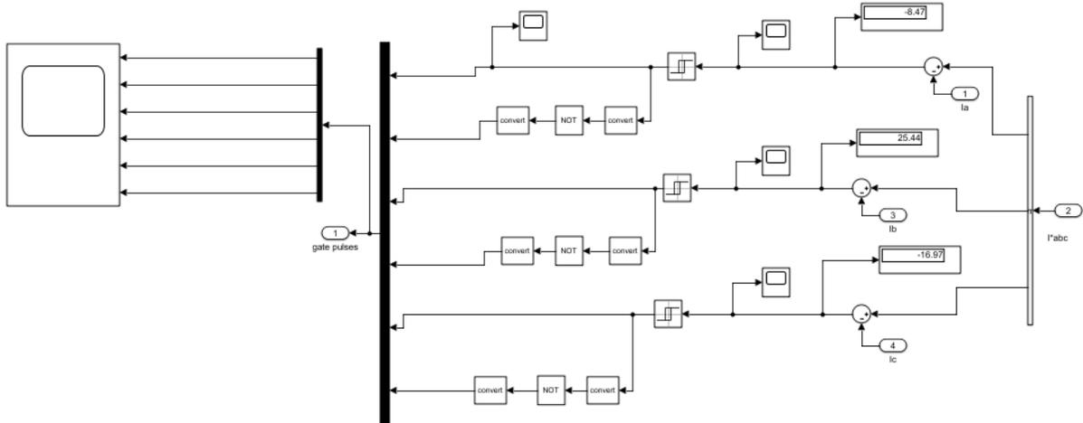
Figure 6 logic circuit for switching of BLDC motor
