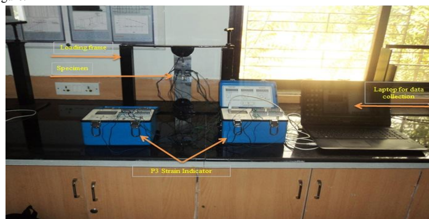
Figure 1:Experimental setup for elliptical cutout (Electrical Strain Gauge Method)
