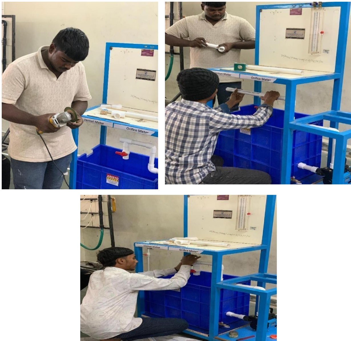
Fig.3.1 GRINDING & PVC PIPE FITTING
