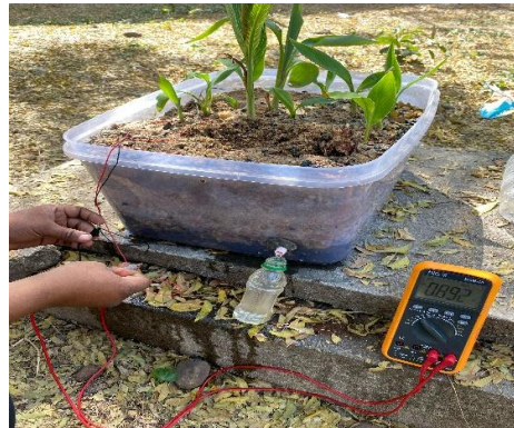
Fig ii: Obtained voltage from MFCs
