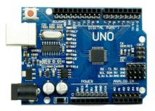
The Arduino Uno is a microcontroller board. it is developed by Arduino Company. It have sets of digital and analog input/output pins it is easy to use for beginners. The Arduino can be powered by USB cable.
