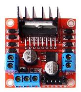
The L299N motor driver control speed and Direction of DC electric motor. The L298N motor driver can control 1/2 motor. It is used in robotics and any other projects. It have inbuilt heat sink to cooling just like a fan it is also known as cooling device. It is made by thermally conducting material.
