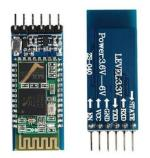
Jaap Haartsen they invited this Bluetooth. The HC 05 Module is used to wireless communication. It is pair with Smart Phone, Tablet etc. with use of this module we transfer the UART data. It can design easily. It is communicate with the help of radio waves. The HC-05 Bluetooth consist Master/Slave Configuration. It allows to make changing setting and configuring the module AT commands.
