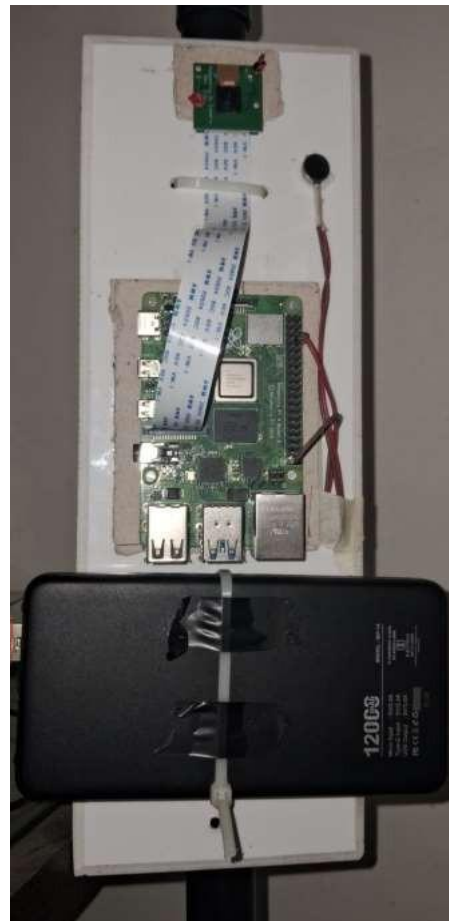
Fig. 7 Prototype of Object Detection System
