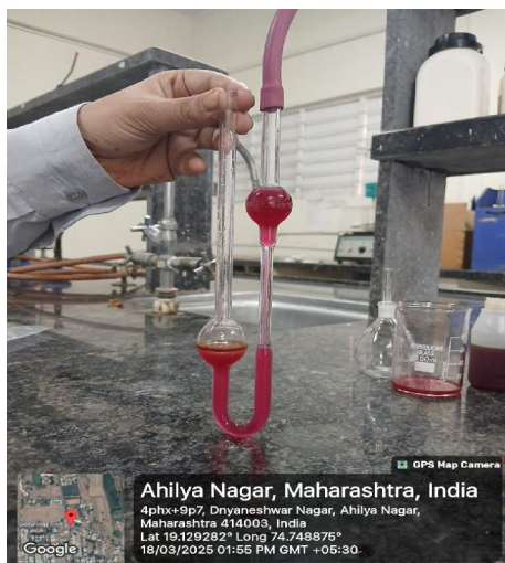
Fig.17. Viscosity of syrup measure by Ostwald viscometer
