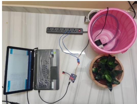
Figure 12: Timer module with Plant Setup
