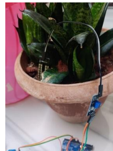
Figure 57: Setup for Soil Moisture sensor
