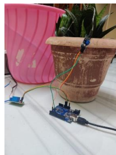
Figure 57: Setup for Soil Moisture sensor
