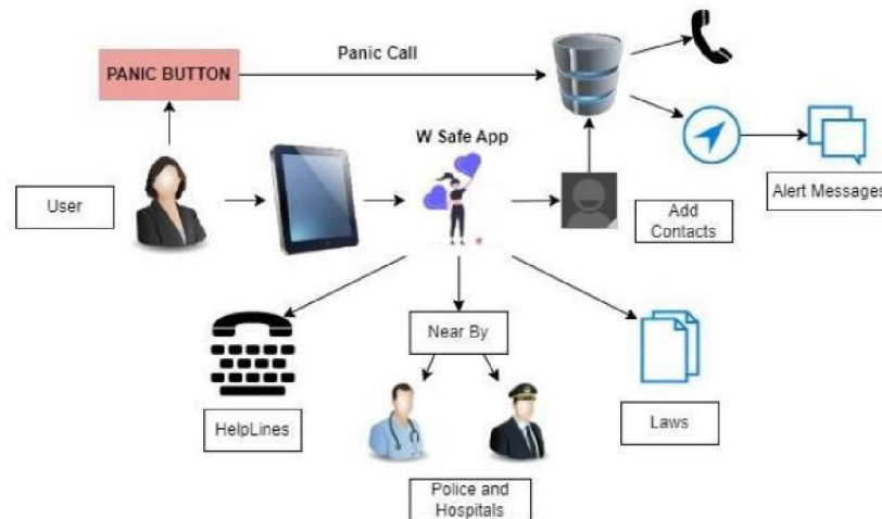
Fig. 1. Her Safety Network System Architecture Diagram.
