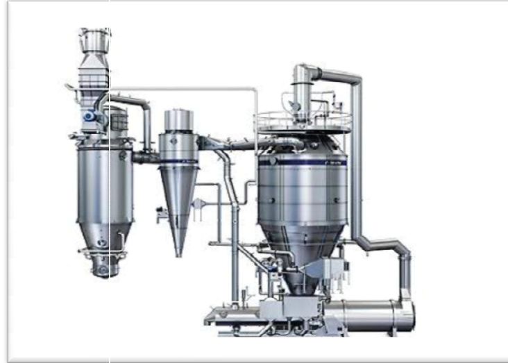
Fig no. 4[Spray Dryer]
