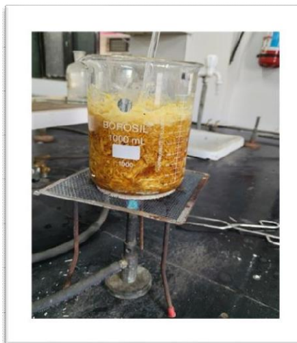
Fig 2. Cooking Bagasse with 10% caustic soda
